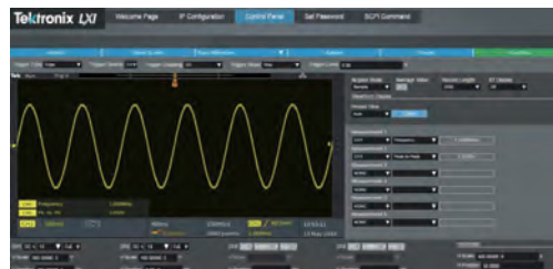
Built-in web page enables remote control of horizontal and vertical scale, trigger settings, and measurements.
