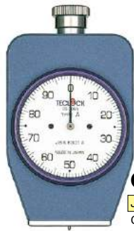
GS-703N JIS C (old type) Hard rubber Ebonite
