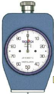
GS-703N JIS C (old type) Hard rubber Ebonite
