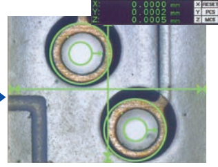
(3) When the two cross-hairs coincide and the target view appears, press the Enter button to complete the measurement.
