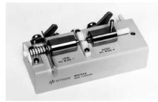
Terminal connector: 4-Terminal Pair, BNC DUT connection: 2-Terminal Dimensions (approx.): 128 (W) x 60 (H) x 71 (D) [mm] Weight (approx.): 270 g Additional error:
