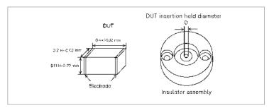
The 16196D is furnished with two different insulator assemblies, since any gaps between the DUT and the cylindrical insulator will result in improper positioning and subsequent measurement errors. Select an insulator assembly that reduces the gap the most. See the table below for dimensions of the insulator assemblies.
