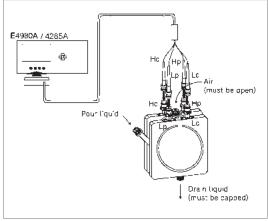
**Compensation and measurement:** Short compensation is recommended in combination with the cable length compensation before measurement. First, set the instrument's cable length compensation function to 1 m. Then, short compensation is performed by using the furnished shorting plate. Open compensation is not performed, but its values are used in the dielectric constant equation as shown below:
