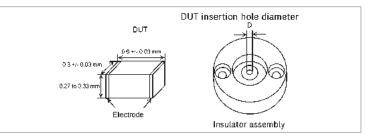
The 16196C is furnished with one insulator assembly. See the table below for the dimensions of the insulator assembly.
