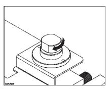
Replace the cap by screwing tightly
