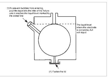
Pouring the liquid into the fixture
