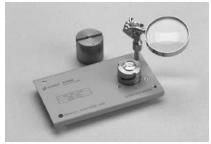
Terminal connector: 7 mm DUT connection: 2-Terminal Electrical length: 26.2 mm Dimensions (approx.): 140 (W) x 48 (H) x 78 (D) [mm] Weight (approx.): 250 g Additional error:
