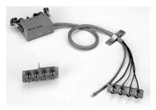
Terminal connector: 4-Terminal pair, BNC Cable length (approx.): 1 m Cable tip: BNC (female) Weight (approx.): 460 g Additional error: For detailed information, refer to the operation manual or the specifications of E4990A. **Description:** The test leads extend the measurement port with a 4-Terminal Pair configuration. It is provided with a BNC male connector board to allow the attachment of user-fabricated test fixtures.
