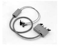
Terminal connector: 4-Terminal Pair, BNC DUT connection: 4-Terminal Cable length (approx.): 1.3 m (from connector to clip's tip) Weight (approx.): 300 g Additional error: The additional error is negligible when compared to the instrument's accuracy. **Description:** This test fixture makes it possible to measure odd-shaped components that cannot be measured with conventional fixtures. It is equipped with two insulated Kelvin clips.
