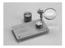
Terminal connector: 7 mm DUT connection: 2-Terminal Electrical length: 26.9 mm Dimensions (approx.): 140 (W) x 48 (H) x 78 (D) [mm] Weight (approx.): 250 g Additional error:
