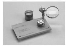
Terminal connector: 7 mm DUT connection: 2-Terminal Electrical length: 27.1 mm Dimensions (approx.): 140 (W) x 48 (H) x 78 (D) [mm] Weight (approx.): 250 g Additional error:
