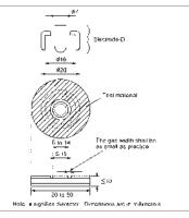
Electrodes for contacting electrode method (Thin Film Electrode)
