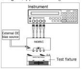
**Description:** This test fixture makes it possible to measure a DUT with up to ±200 V DC bias. The same modules of 16047A can be used to allow measurements of axial/radial lead components.
