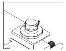
Remove the cap of the fixture
