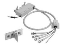
Terminal connector: 4-Terminal Pair, BNC Cable length (approx.): 0.94 m (from connector to cable tip) Cable tip: BNC (male) Weight (approx.): 315 g Additional error: For detailed information, refer to the measurement instrument's specifications. **Description:** The test leads extend the measurement port with a 4-Terminal Pair configuration. It is provided with a BNC female connector board to allow the attachment of user-fabricated test fixtures.
