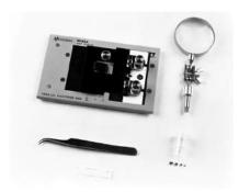
Terminal connector: 7 mm DUT connection: 2-Terminal Electrical length: 11 mm Dimensions (approx.): 150 (W) x 70 (H) x 90 (D) [mm] Weight (approx.): 400 g Additional error:
