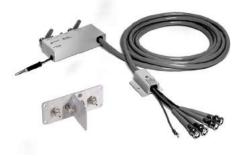
Terminal connector: 4-Terminal Pair, BNC Cable length (approx.): 3.8 m (from connector to cable tip) Cable tip: BNC (male) Weight (approx.): 690 g Additional Error: For detailed information, refer to the measurement instrument's specifications. **Description:** The test leads extend the measurement port with a 4-Terminal Pair configuration. It is provided with a BNC female connector board to allow the attachment of user-fabricated test fixtures. **Applicable instruments:** E4980A/AL
