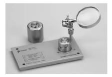
Terminal connector: 7 mm DUt connection: 2-Terminal Electrical length: 27.3 mm Dimensions (approx.): 140 (W) x 48 (H) x 78 (D) [mm] Weight (approx.): 250 g Additional error:
