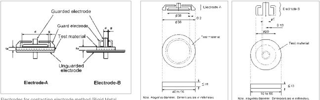
Electrodes for contacting electrode method (Rigid Metal Electrode)
