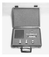
Terminal connector: 7 mm Dimensions (approx.): 350 (W) x 100 (H) x 270 (D) [mm] Weight (approx.): 2.0 kg **Description:** The 16190B is a performance test kit designed to verify the impedance measurement accuracy of LCR meters or impedance analyzers that have a 7 mm measurement terminal. Refer to the instrument's operation/service manual for the method of using these standards.
