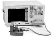
**Description:** The 16451B is used to evaluate the dielectric constant of solid dielectric materials accurately, and complies with ASTM D150. The 16451B employs the parallel plate method, which sandwiches the material between two electrodes to form a capacitor. LCR meter or an Impedance Analyzer is then used to measure the capacitance created from the fixture. A measurement block diagram of the parallel plate method is shown below:
