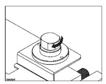
Replace the cap by screwing tightly
