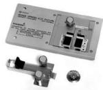
Terminal connector: 7 mm DUT connection: 2-Terminal Electrical length: 3.4 mm Dimensions (approx.): 150 (W) x 70 (H) x 80 (D) [mm] Weight (approx.): 180 g Additional error: See figure below
