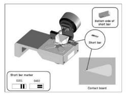
**Description:** This test fixture is designed for impedance evaluations of bottom electrode SMDs. It achieves stable frequency characteristics up to 3 GHz and provides highly repeatable measurements. This test fixture supports two SMD sizes, 0201 (mm)/ 008004 (inch) and 0402 (mm)/01005 (inch).
