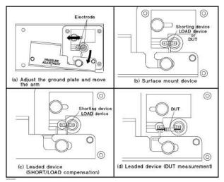
Placing the device
