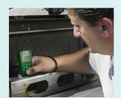
Extech's CG104 offers a quick, one-handed operation, non-destructive measurement of the thickness of ferrous and non-ferrous substrates. Its unique reversible display allows you to take readings in challenging angles of area being measured.
