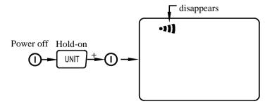
When the meter is normally turned on, the audible sound function is on.
